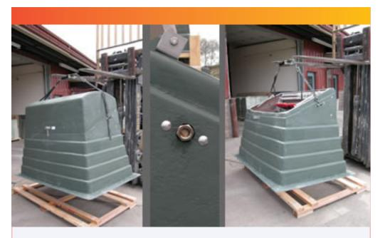
New lifting nuts now standard on all direct buried and padmount Cable Junction Pedestals. A 5/8-11 SS nut is welded to a SS backing plate which is bolted to the pedestal wall on both sides. This allows the pedestal to be lifted the same way a single phase transformer is slung. The blind nut is positioned to lift uniformly whether the top is on or off. The lifting eye bolts near the bottom are no longer provided.
